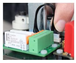
Clip the relay board with the spacers in the locating holes. Connect the main board with the connection cable. Connect according to the wiring diagram.
