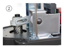
Place the bracket with the lever over the ball pin and screw it tight.
