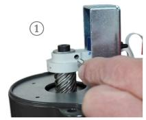
Screw the ball pin in the drilled hole of the magnet holder by using an open-end wrench (size 5,5 mm).
