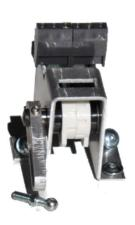
1 pre-assembled bracket with limit switch board, switching cams and lever, 1 ball pin, 3 screws Standard switches 2WE: silver/nickel contacts, current: 0,1 A to 5 A, voltage: 24 V to 230 V. Optional 2WE gold: gold contacts, current 0, 1mA to 100 mA, voltage: 5 V to 24 V
