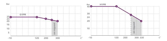
\*For temperature above 100℃ a compensation chamber is needed.
