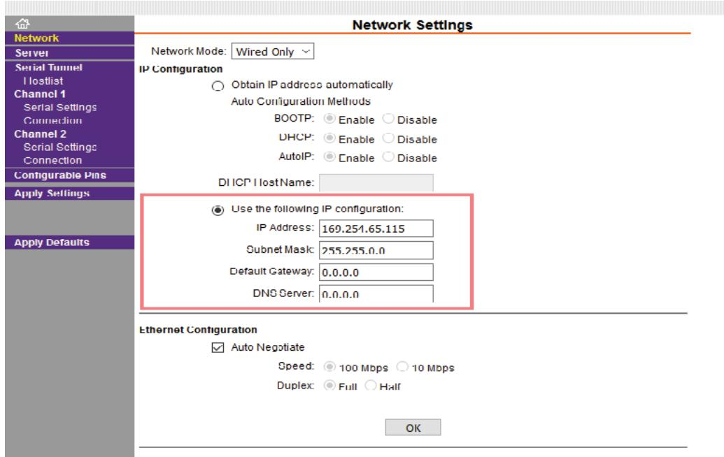
Under "IP Configuration", assign a fixed IP address for the device and enter the subnet mask. Confirm the settings with OK.
