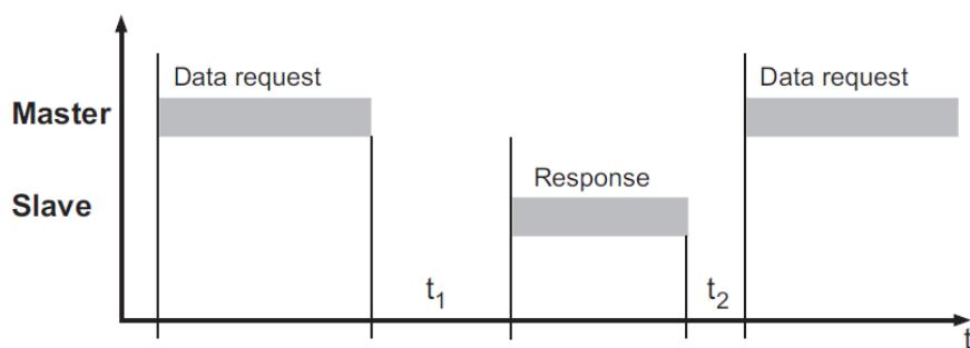
The data request and response consist of several characters (each with a start bit, 8 data bits, a parity bit if necessary, and a stop bit) which are transmitted coherently.
