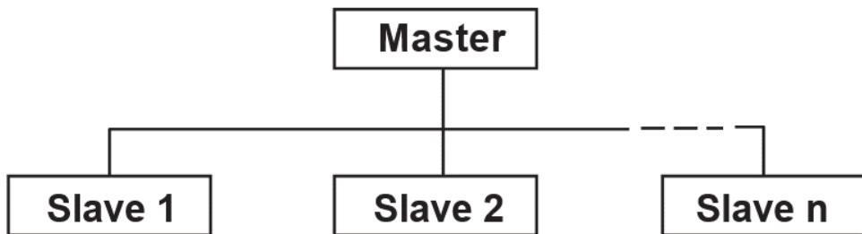
The master controls the data exchange; the slaves only have a response function. They are identified by their device address.
