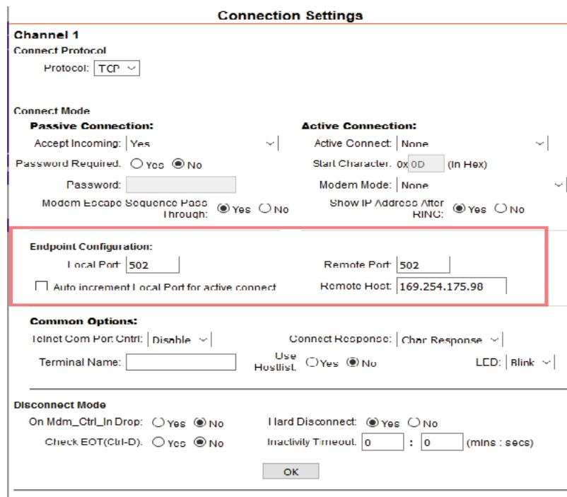
Under "Endpoint configuration", enter the IP address of the Modbus master in the "remote host" field. Enter the port number 502 into the two fields "local port" and "remote port". Confirm the settings with OK. *(All necessary settings have now been made)*
