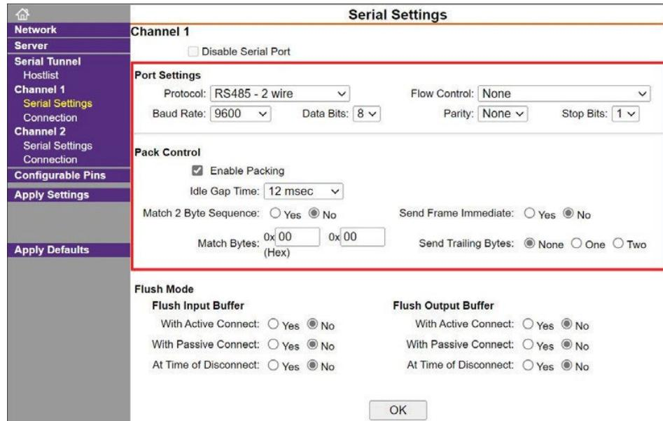
If necessary, change the values under "Port Settings" and "Pack Control" so that they match the settings in this figure. Confirm the settings with OK.
